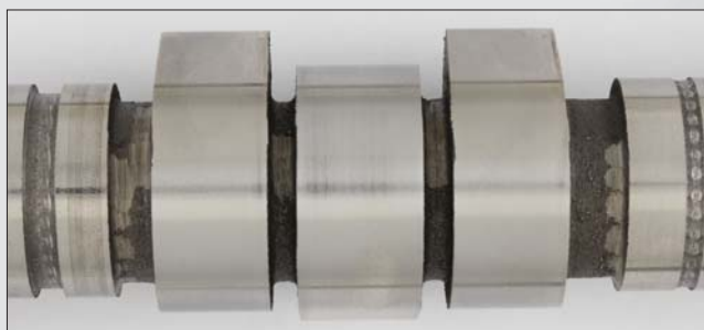
After rigorous third-party testing, the cam lobes show little-to-no wear.
